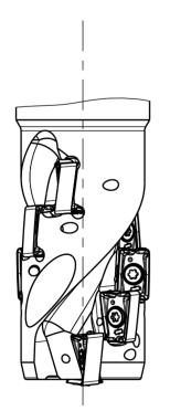
BALANCE GRADE PER DIN ISO 21940-11 G 6.3 / 3000 min<sup>-1</sup> MASS APPROX. 0.6 kg
